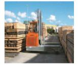
protruding loads such as timber, steel rods, pipes, etc. Trucks can be powered by battery, LPG or diesel and may have 3 or 4 wheels depending on the requirement. Commonly, loads of about 5,000 kg can be lifted to heights of 8 metres, but specialist trucks with a capacity of 50,000 kg are available.
