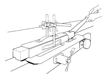
Figure 4 A push stick in use at a woodworking machine
